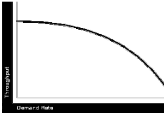
Figure 23-4: Increased Response Time/Reduced Throughput
